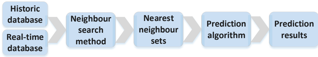
Figure 3.3 : Processing flow of the ST-kNN algorithm.
