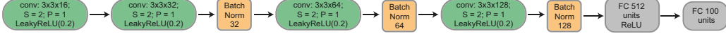
Figure 4.4: The structure of \phi_\omega in MMD-D on MNIST . The kernel size of each convolutional layer is 3; stride (S) is set to 2; padding (P) is set to 1. We do not use dropout. Best viewed zoomed in.
