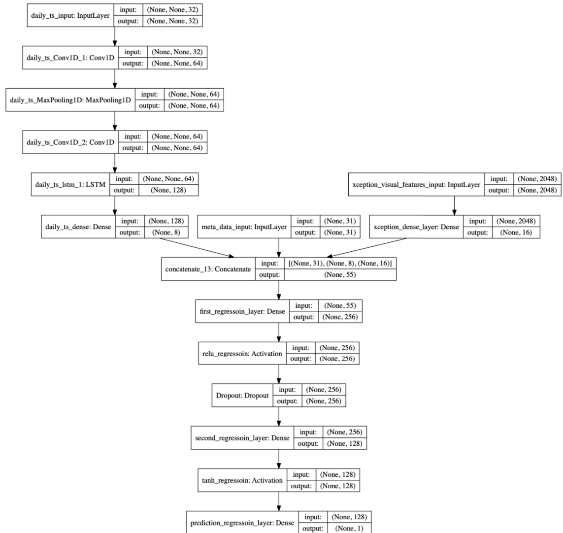
Figure 6.22: Visual base prediction model based on Xception visual feature extraction and daily adjusted median price (Conv1D + LSTM)
