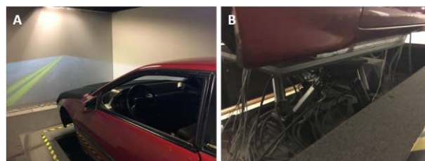
Fig. 2.4 Simulated driving setup: (A) the mimicking highway scenario; (B) the maneuvering platform with installed converted car.
