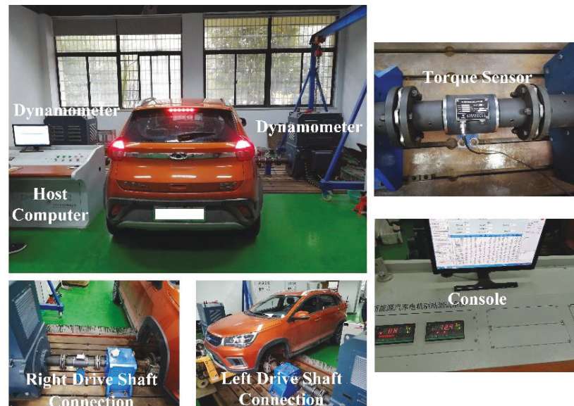
Figure 6.9 Experiment for Drive Shaft Torque Observation
