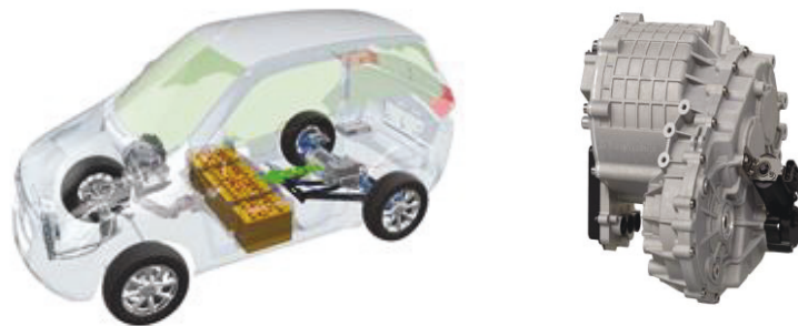
Figure 1.4 Typical Centralized Driven Electric Vehicle Powertrain Layout
