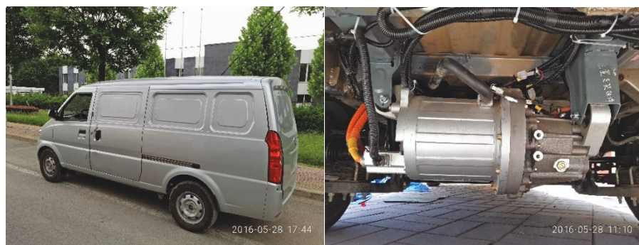
Figure 1.6 Electric Logistics Vehicle Prototype with Integrated Powertrain
