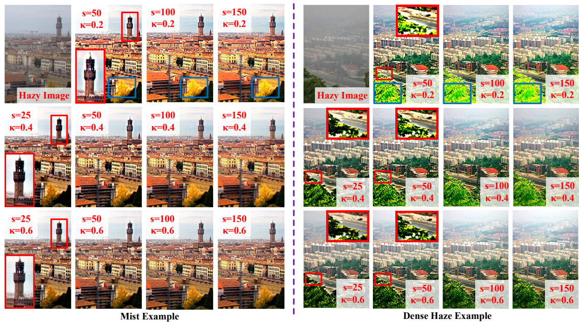
Figure 4.5: Image dehazing using VROHI with different combinations of s and \kappa while \omega is fixed at 0.95 and \theta is fixed at 0.103.
