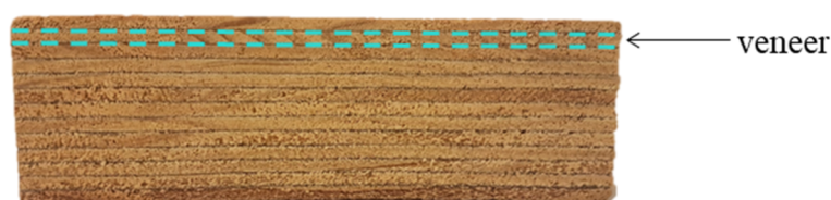
Figure 3-3 Cross-section of LVL showing veneers
