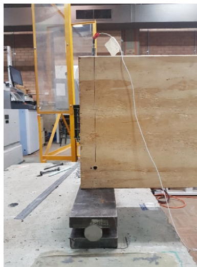
Figure 4-3 Steel shaft and plate pin boundary condition
