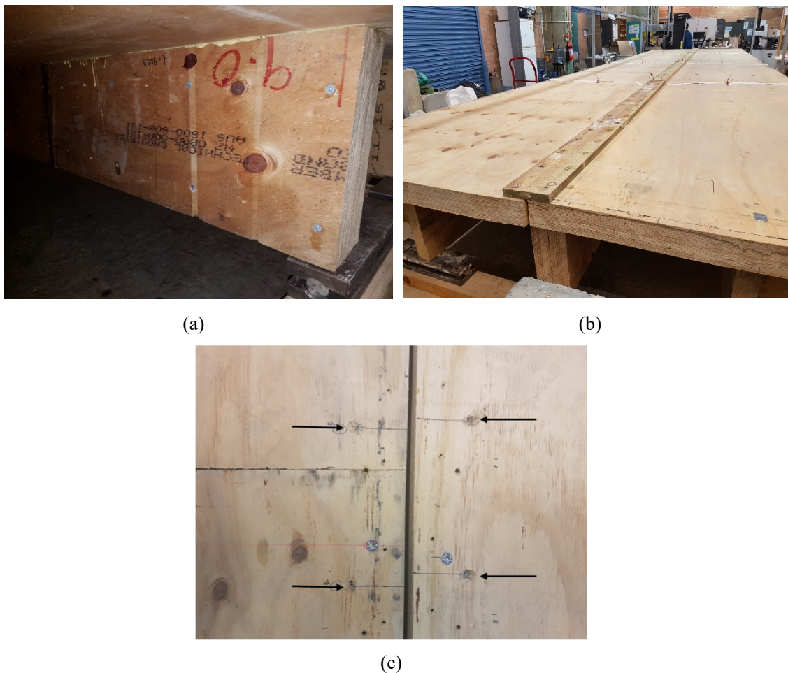
Figure 6-29 Photo of (a) web-to-web connection at 300 mm c/c; (b) splice connection between flanges with screws at 150 mm c/c; (c) plan view of diagonal screw connections at 150 mm c/c (arrows indicate screw locations).
