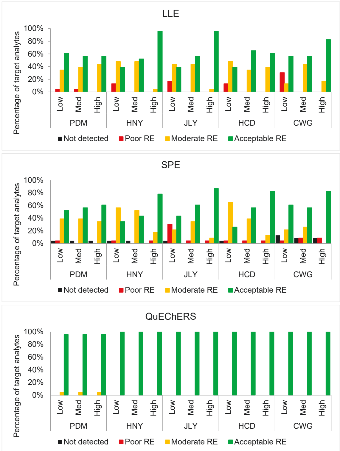
Fig. 3.5.2B: The extraction recovery (RE) of liquid-liquid extraction (LLE); solid-phase extraction (SPE); and modified quick, easy, cheap, effective, rugged, and safe (QuEChERS) at low (0.1 µg/mL); medium (Med, 0.4 µg/mL); and high (1 µg/mL) quality control levels. Note: RE category: acceptable ( \pm 25\% ), moderate ( \pm 25\% to \pm 75\% ), and poor (less than -75\% or more than +75\% ) (Abbreviations: PDM, powdered drink mix; HNY, honey; JLY, jelly; HCD, hard candy; CWG, chewing gum)
