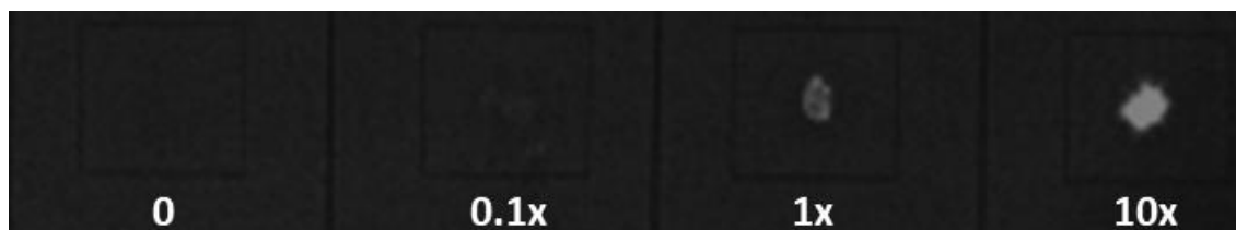
Figure 23: MDA placebo with Gel Red® at concentrations between 0 and 10x spotted onto copy paper and imaged with the Molecular Imager® Gel Doc™ XR under short wavelength UV
