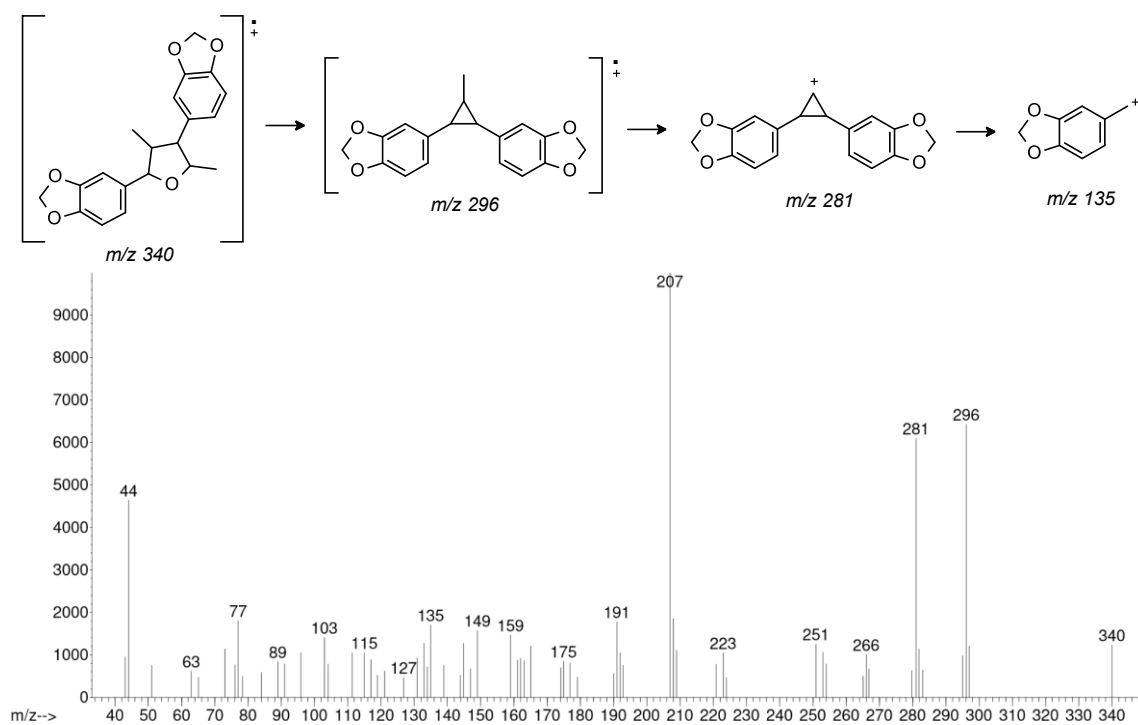
Figure A1-4: Mass spectrum and proposed fragmentation scheme of organic impurity 22
