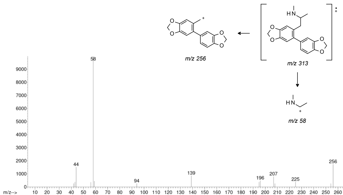
Figure A1-29: Mass spectrum and proposed fragmentation scheme of organic impurity 74
