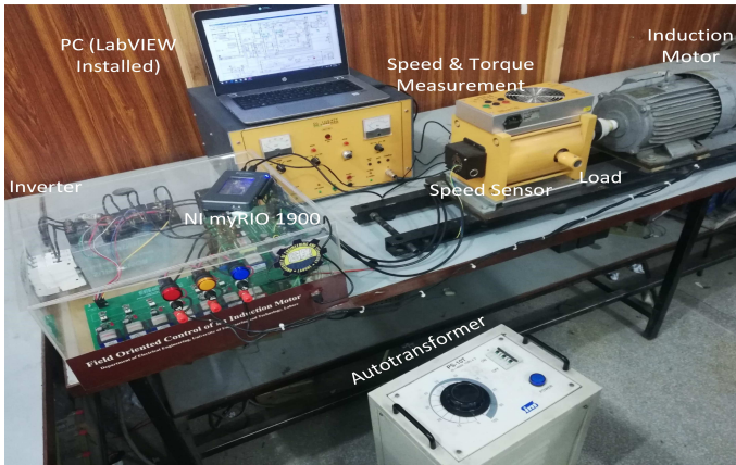
Fig. 10: Induction machine based electrical drive setup
