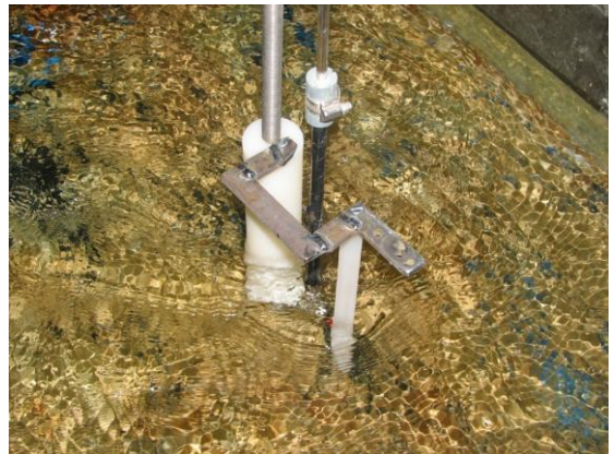
Figure 3.4. Photographs of measuring velocity components by ADV; a) control test; b) test with d/D=1.5
