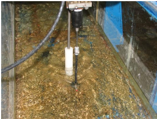
Figure 3.4. Photographs of measuring velocity components by ADV; a) control test; b) test with d/D=1.5
