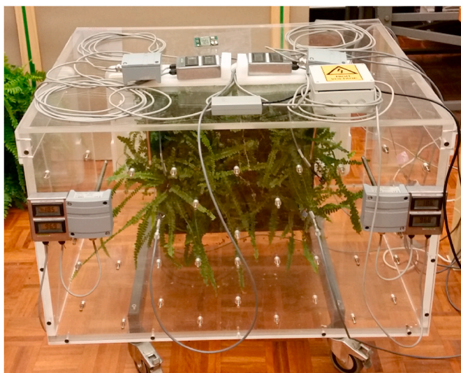
Fig. 2. Acrylic-sheets chamber with a green wall module ( Nephrolepis cordifolia ). (For interpretation of the references to colour in this figure legend, the reader is referred to the Web version of this article.)
