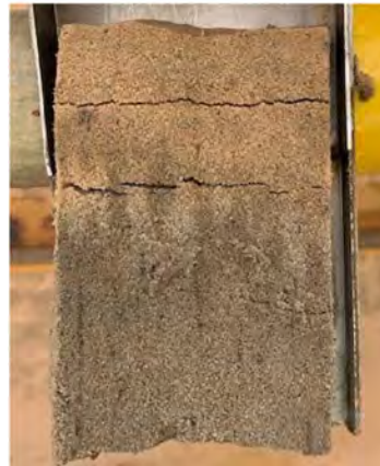
Figure 1: A sample of the track profile which is failed based on the sand profile inspection criteria. Due to the confidentiality purposed, the name of the track is not revealed.
