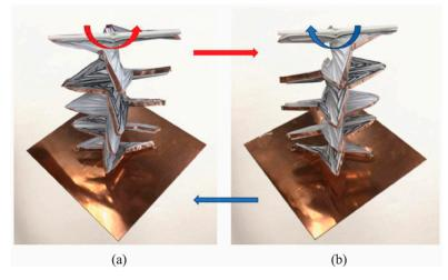
**Figure 7.** The prototype of the bifilar segmented helical antennas at (**a**) left-handed and (**b**) right-handed angles [103].
