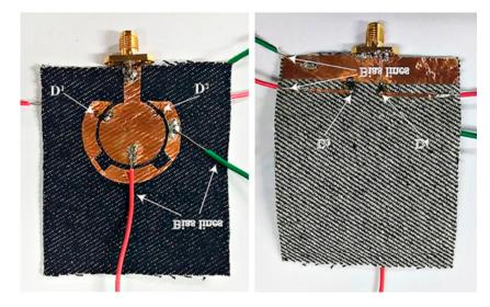
**Figure 8.** Fabricated prototype of the frequency and polarization-reconfigurable antenna on jean substrate in [109].
