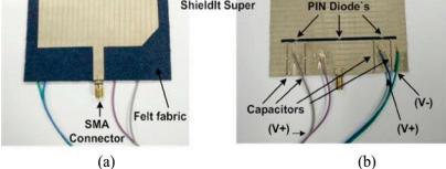
**Figure 9.** The fabricated frequency-reconfigurable antenna based on textile in [1]: (**a**) front view; (**b**) back view.
