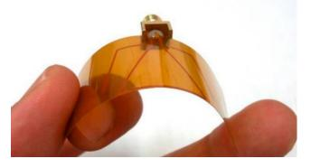
Figure 4. Fabricated prototype of the pattern-reconfigurable antenna on flexible polyimide in [85].
