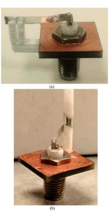
**Figure 10.** Pattern and frequency-reconfigurable antenna based on liquid crystalline elastomers: (a) straight statues; (b) helix structure with 1.1-turn [113].
