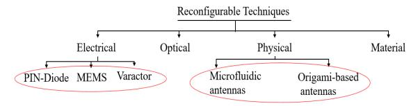
Figure 1. Categorization of reconfiguration techniques for all types of antennas.
