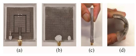
**Figure 2.** The fabricated frequency-reconfigurable antenna on polydimethylsiloxane (PDMS) substrate in [24]: (a) front view; (b) back view; (c) side view; (d) bending position.
