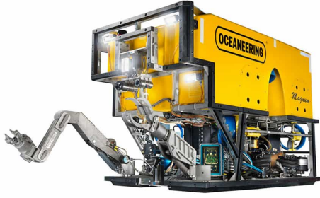
(a) The Magnum Plus ROV from Oceaneering
