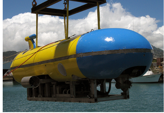
(b) The Semi Autonomous Vehicle for Intervention Missions (SAUVIM) from the Autonomous System Laboratory of the University of Hawaii
