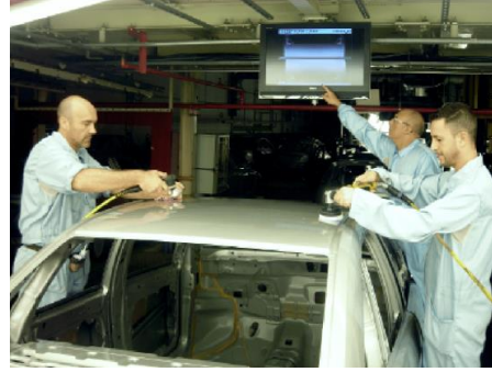
(b) Fixing defects identified by a visual detection system in a Ford automotive plant [Armesto et al. , 2011].
