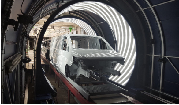
(a) Inspection light tunnel system in a Mercedes automotive plant [Munoz et al. , 2019].
