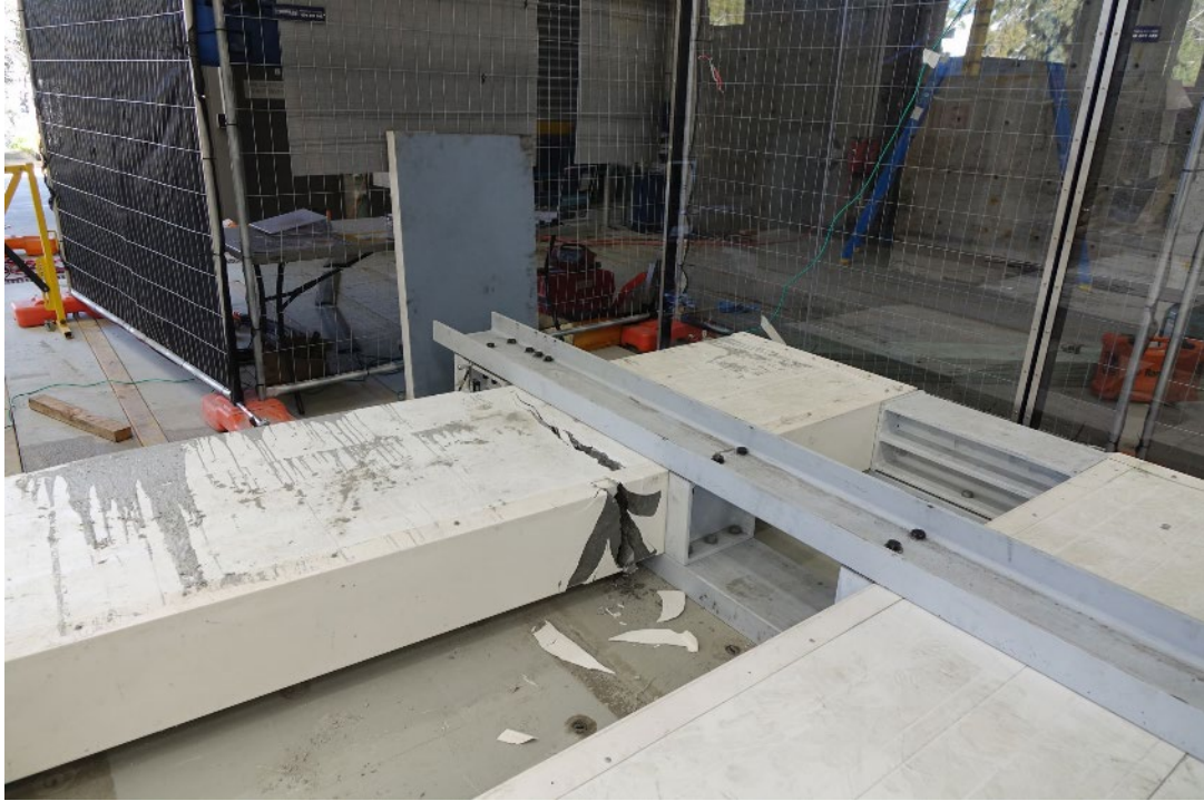
Figure 8. Failure mode of the walls under compressive lateral loads
