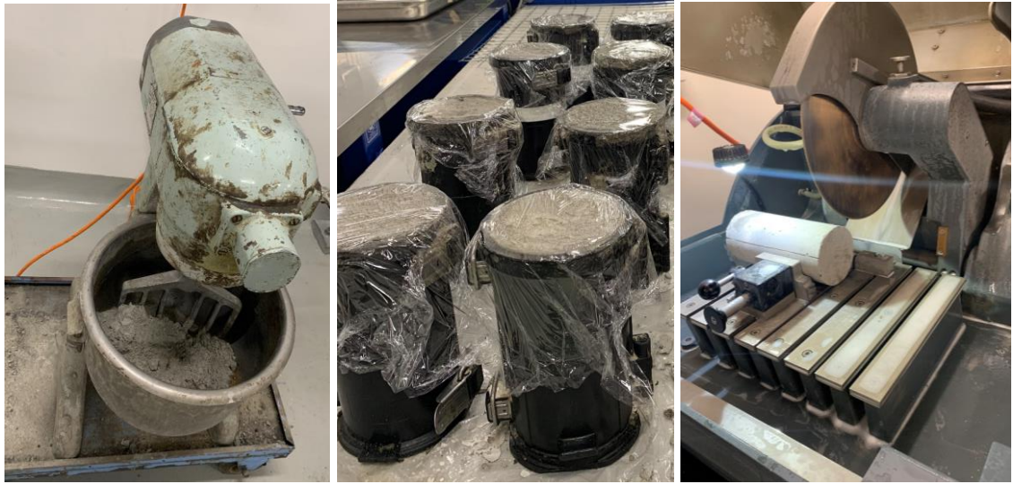
Pic. S5.1. Concrete casting and slicing
