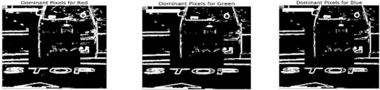
(b) Dominant pixels for the respective R, G and B color spaces of a day image
