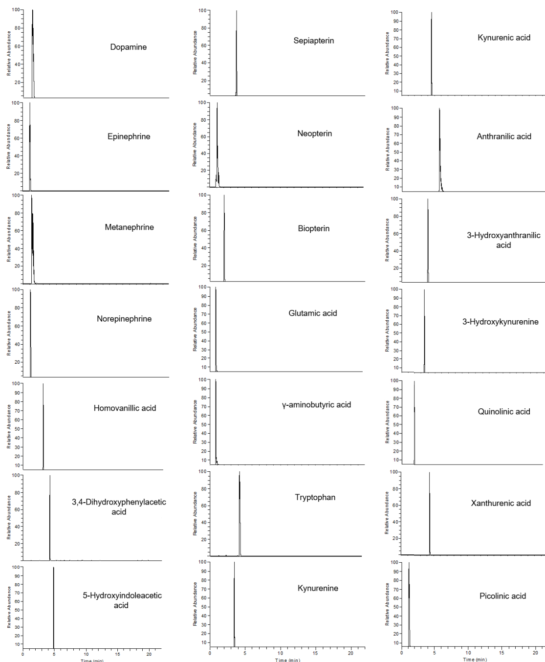
Figure 2-4 Extracted ion chromatograms of metabolites in pooled CSF using Waters HSS T3 Column on the Thermo Scientific Vanquish system coupled to a Q Exactive HF-X Hybrid Quadrupole Orbitrap Mass Spectrometer. Metabolites were confirmed using reference standards.
