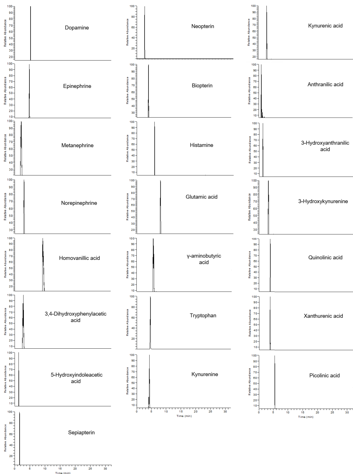
Figure 2-5 Extracted ion chromatograms of metabolites in pooled CSF using Agilent HILIC Column on the Thermo Scientific Vanquish system coupled to a Q Exactive HF-X Hybrid Quadrupole Orbitrap Mass Spectrometer. Metabolites were confirmed using reference standards.
