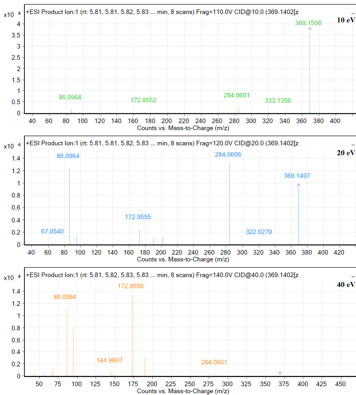
Figure A2-20: MS/MS spectra obtained from AH-7959
