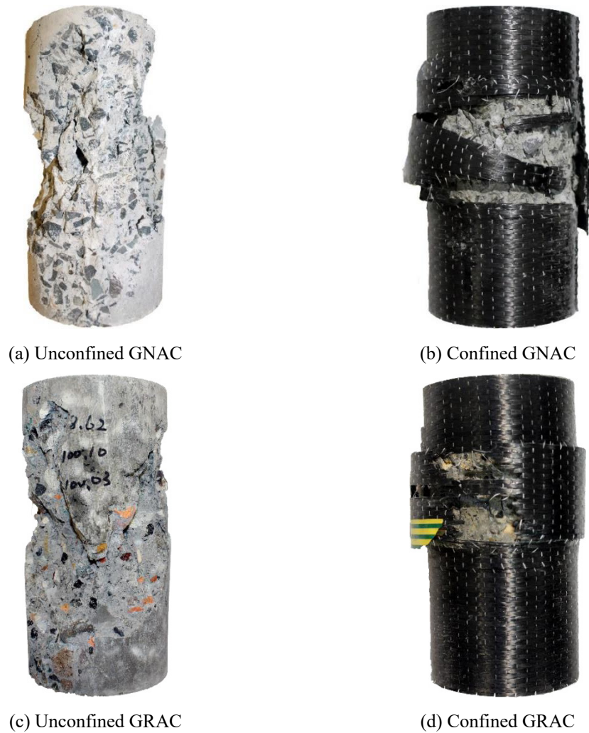
Figure 7.3. Typical failure modes of specimens under compression
