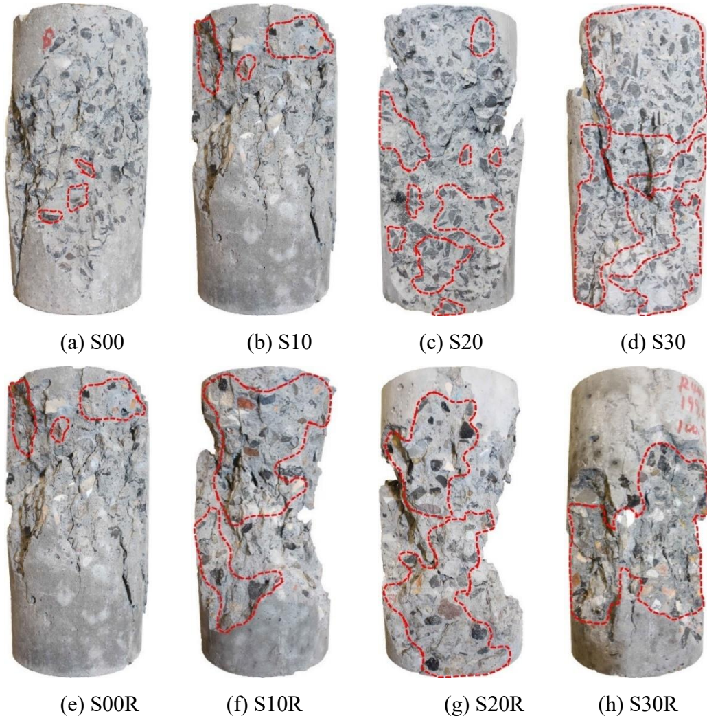
Figure 5.3. Failure patterns of geopolymeric concrete under quasi-static loading(fractured aggregate particles marked within red lines)
