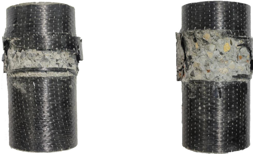
(a) Replacement ratio of 0%, number of CFRP layers of 2 (b) Replacement ratio of 100%, number of CFRP layers of 2 Figure 8.1. Typical failure modes of CFRP-confined geopolymeric concrete
