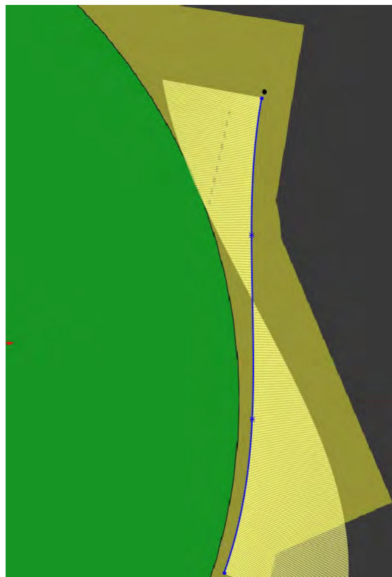
Figure 4: Modelling of greyhound trajectory and associated curvature combs for Design 3 Mandurah greyhound track catching pen run.
