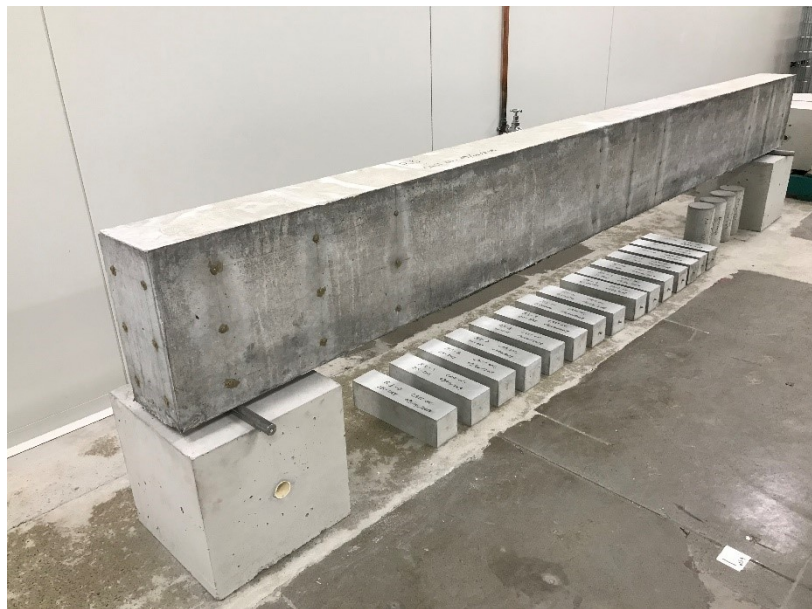
Figure 7. 11 DEMEC points arrangement (R3 beam – reactive reinforced concrete beam)
