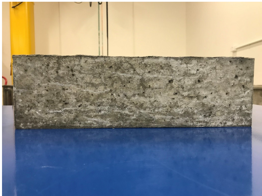
Figure 5. 12 External cracks on reinforced beam after 3 cycles in the autoclave
