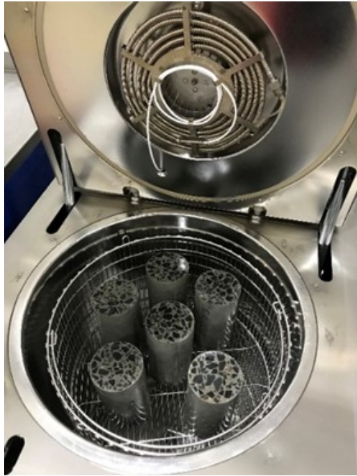
Figure 3. 7 Non-reactive concrete cylinders (90-day) in Zirbus LVSA 50/70 autoclave
