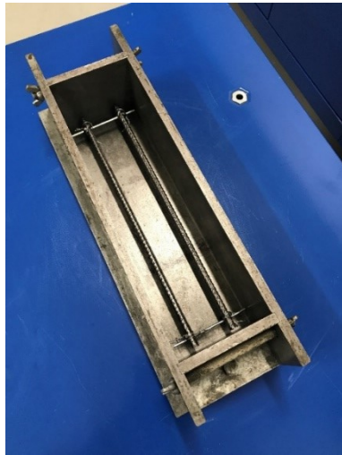
Figure 5. 2 Reinforcing steel bars in steel moulds
