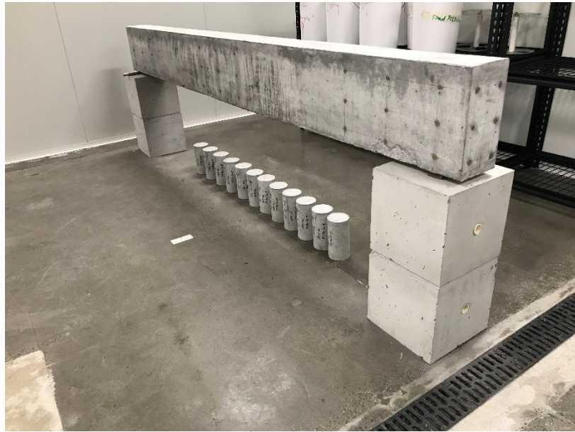
Figure 7. 10 DEMEC points arrangement (R2 beam – reactive reinforced concrete beam)
