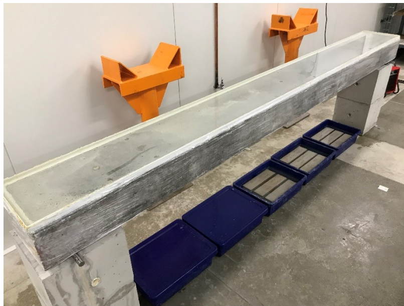
Figure 7. 18 Water supply of R3 beam – reinforced concrete beam (similar set up for R2 and R4 reinforced concrete beams)
