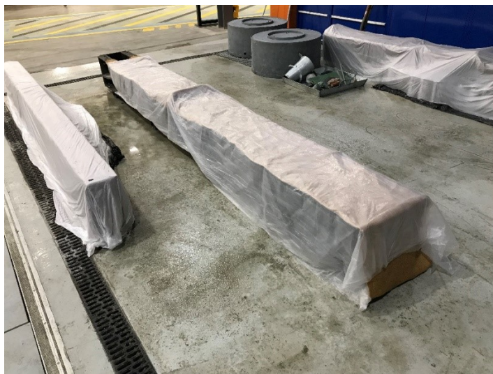
Figure 7. 6 Moist curing of beams and companion specimens in the laboratory at a temperature of 23 \pm 2 \text{ }^\circ\text{C}
