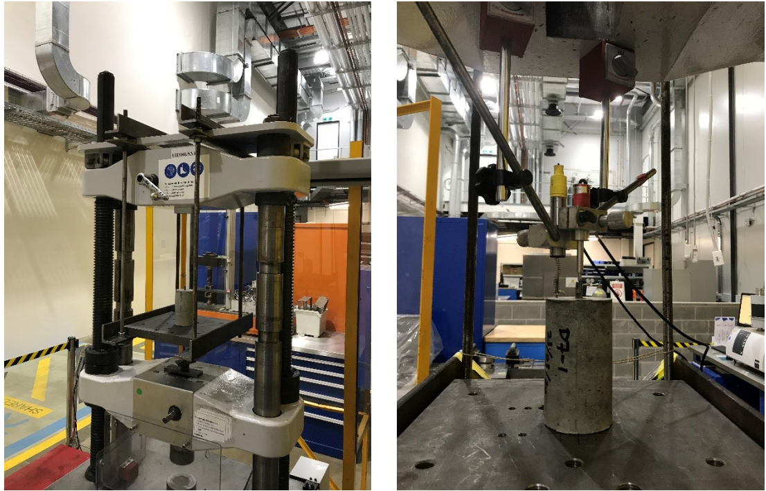
Figure 6. 14 Instrumentation and test set-up for the pull-out tests
