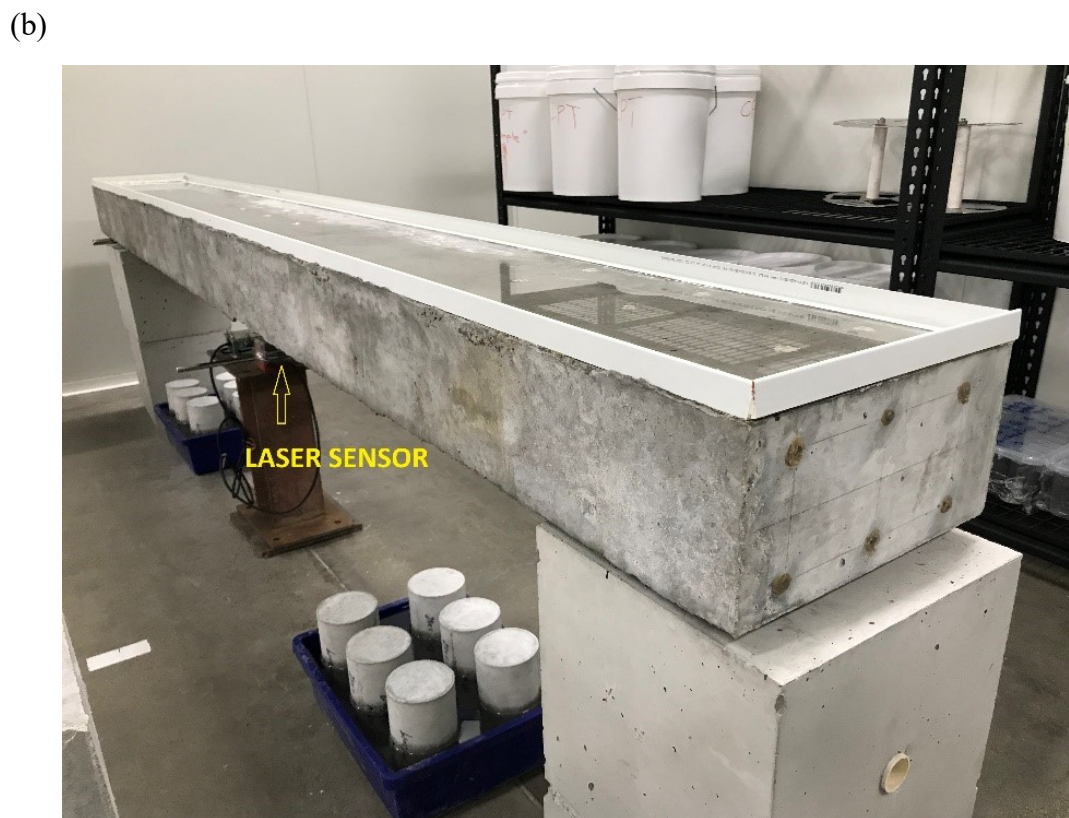
Figure 7. 37 (a) Schematic set-up of laser displacement sensor; (b) Deployment of laser sensor for R2 beam to measure the displacement of the beam
