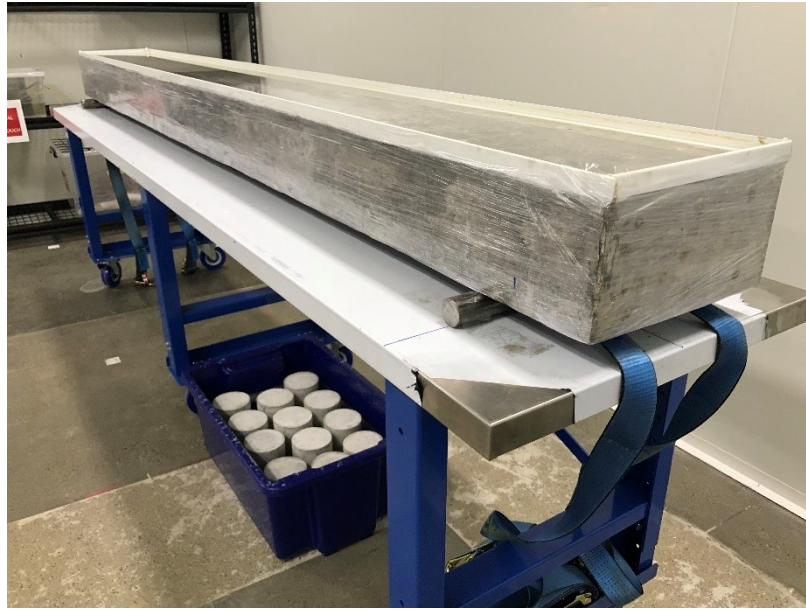
Figure 7. 17 Water supply of R1 beam – plain concrete beam, simply supported
