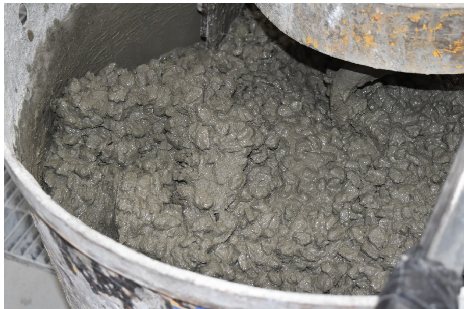
Figure 7. 2 Concrete mixing using a 70L pan mixer
