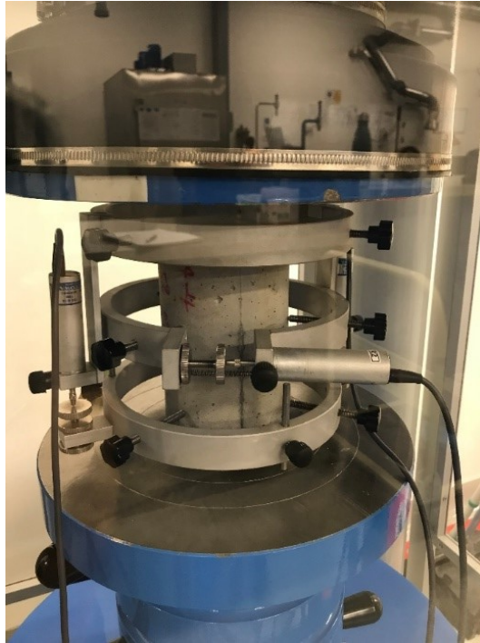
Figure 5. 6 Modulus of elasticity test on 100 mm diameter 200 mm height cylinder
