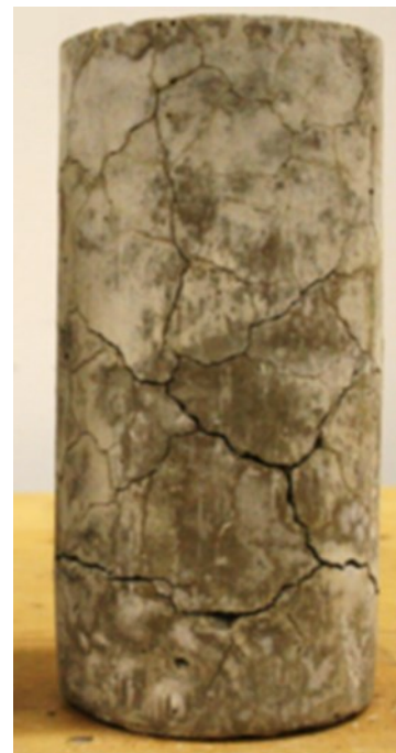
Figure 7. 24 Comparison of cylinders at the age of more than 5 years cured in: (a) fog-room with 100%RH at 23 °C and (b) field exposure conditions (Karthik, Mander & Hurlebaus 2016b)
