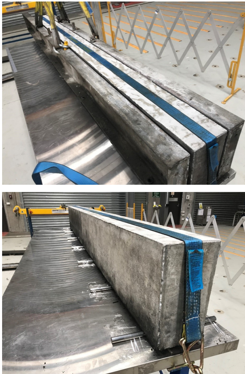
Figure 7. 7 Demolding of R1 beam – reactive plain concrete beam
