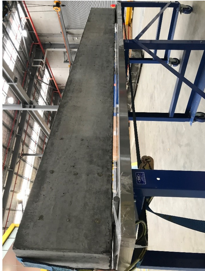
Figure 7. 9 DEMEC points arrangement (R1 beam – reactive plain concrete beam)
