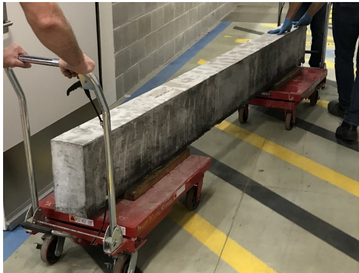
(a) Transporting beam using two trolleys
