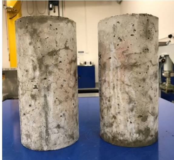
Figure 4. 16 External cracks on cylinder after 3 cycles in the autoclave
