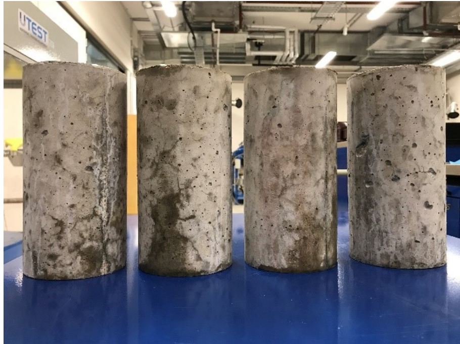
Figure 5. 11 Crack pattern of cylinders after 3 cycles of autoclaving
