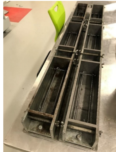
Figure 5. 2 Reinforcing steel bars in steel moulds
