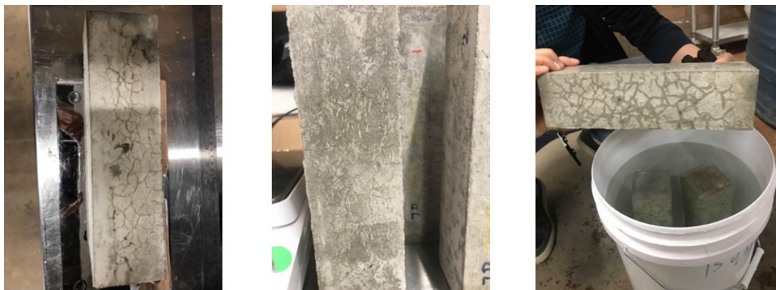
Figure 3. 9 Crack patterns of reactive aggregate B prisms with 3% \text{Na}_2\text{O}_{\text{eq}} boosting after 3 cycles of autoclaving at ages of 3, 7, and 28 days
