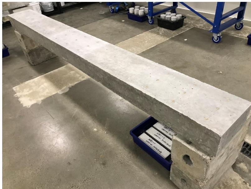
Figure 7. 13 DEMEC points arrangement (NR1 beam, non-reactive reinforced concrete beam, flipped over)
