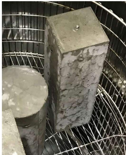
Figure 4. 17 External map cracking on prism after 3 cycles in the autoclave
