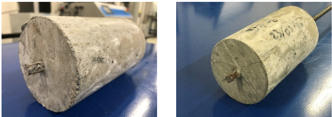
(b) Failure mode of D7-5 and D7-6
