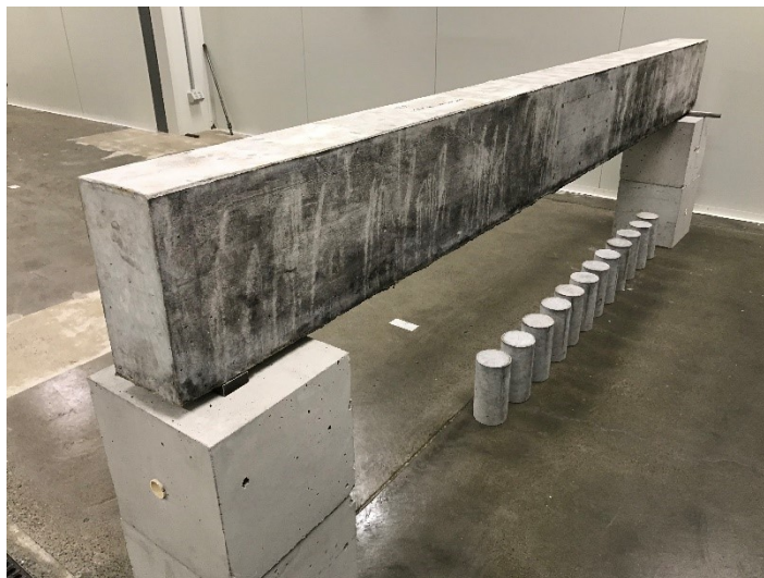
Figure 7. 8 Moving reinforced concrete beam into 38 °C climate chamber
