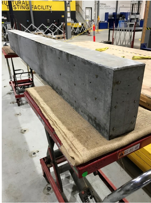
Figure 7. 12 DEMEC points arrangement (R4 beam – reactive reinforced concrete beam)
