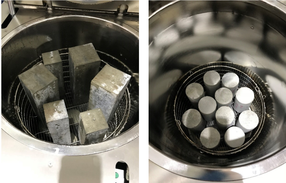
Figure 5. 4 Specimens as placed in the Zirbus LVSA 50/70 autoclave
