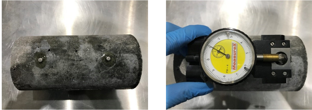
Figure 7. 14 DEMEC points adhered on surface of cylinder and length measurement
