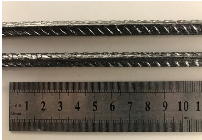
Figure 6. 7 Rib pattern of 8 mm diameter deformed bar
