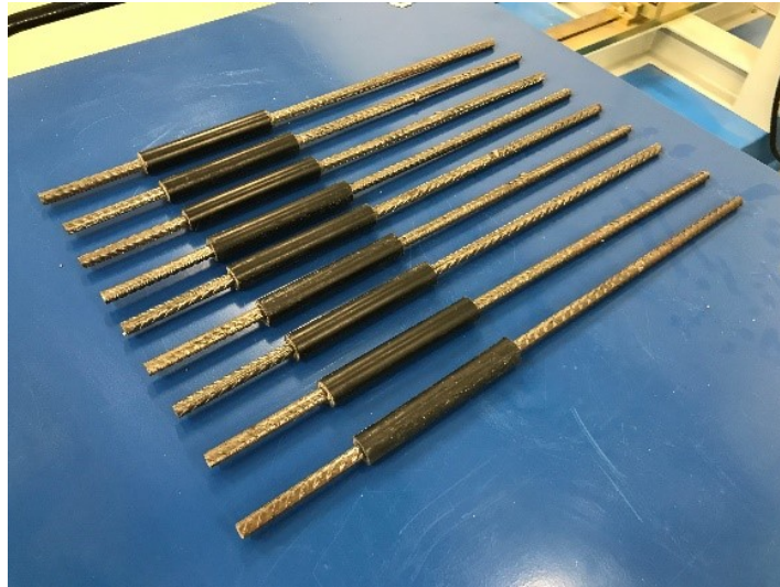
Figure 6. 9 Reinforcing steel bars with 80 mm long tubes
