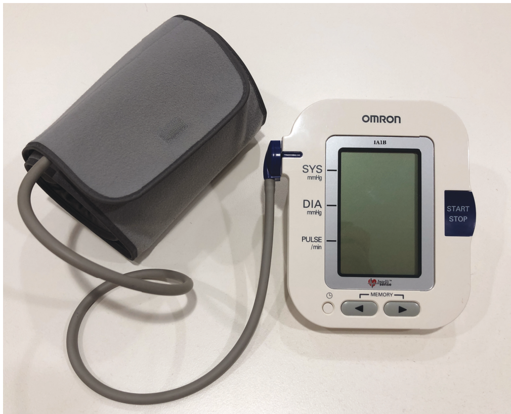
Figure 2.1. The non-invasive automatic blood pressure device used to record participant brachial blood pressure.
