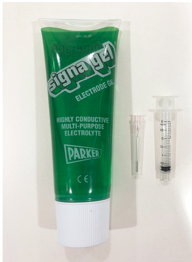
Figure 2.7. Electrode gel used to fill electrodes in the EEG cap, sterile syringe and blunted needle.
