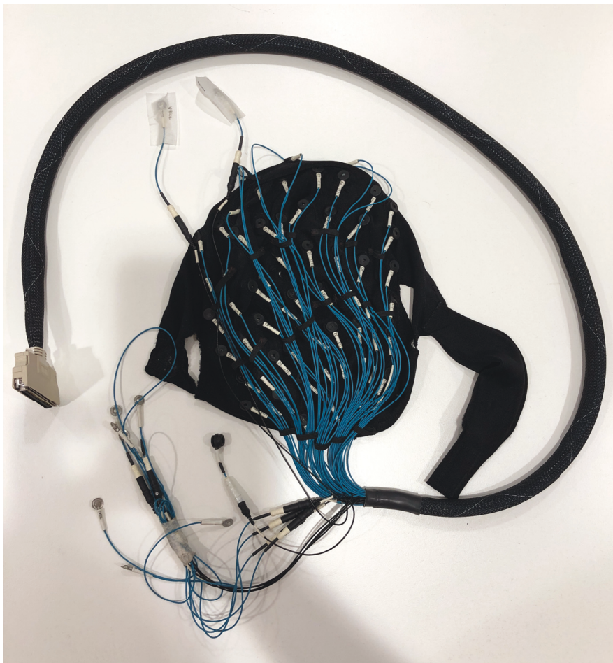
Figure 2.5. The 32-channel non-invasive, elastic EEG cap used to record brain electrical activity from study participants.
