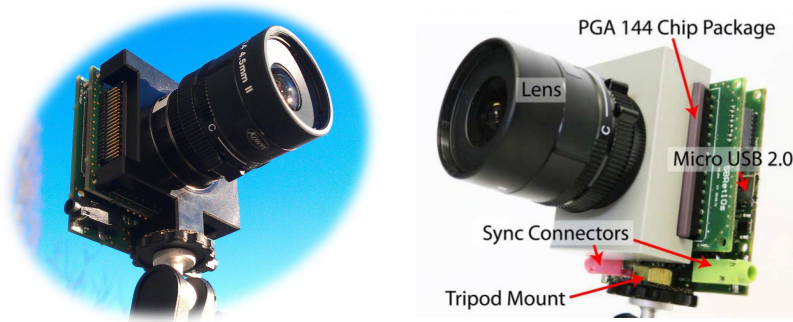
FIGURE 5.1: Pictures of DVS sensors. On the right is the DAVIS240 (image source: inivation.com). On the right is a propototype as shown in [66].
