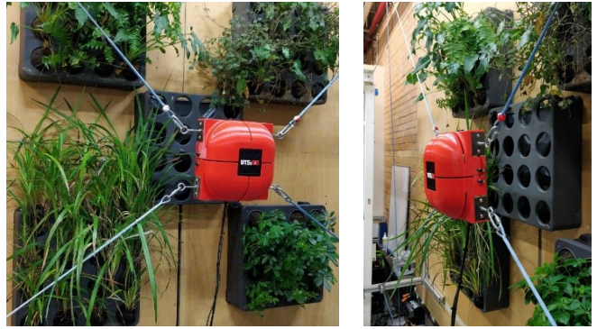
Figure 6: Wallbot being maneuvered across a mock green wall.
