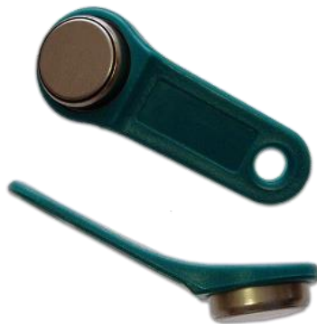
Figure 11. i-Button temperature logger (DS1921G, Thermochron, USA) used in this study, with protective FOB casing for impact protection.
