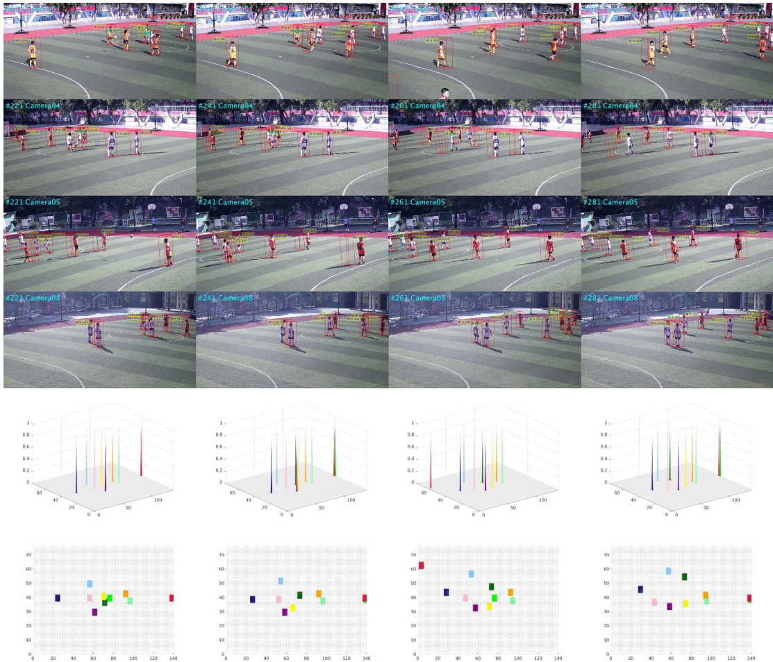
Figure 6.4 : Illustration of our localization results implemented on LH0716v2 dataset. The red cube refers to the generated location, while the yellow label indicates the detected identification outcome. In row No. 5 and 6, different colors refer to unique ID labels. Row No. 5 illustrates the localization results in 3D space, while No. 6 shows the results on the ground plane of bird-eye view.
