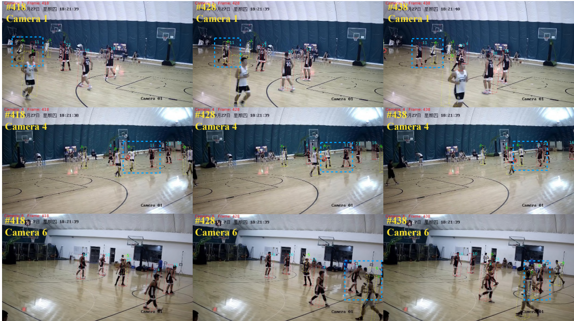
Figure 5.6 : Illustration of our localization results on the STU dataset in Camera 1, 4, and 6. The blue dotted boxes show that our method avoids identity switch between Player 6 of the white team and Player 11 of the black team.
