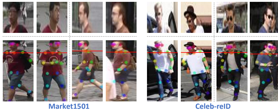
Figure 5.11 : Pose estimation results (the bottom row). The head images (the top row) are extracted according to the location of keypoint of the neck.
