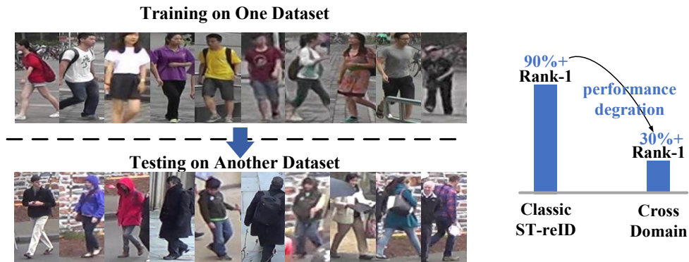
Figure 1.3 : Schematic diagram of cross-domain ST-reID. It can be seen that compared with the single-domain ST-reID issue in which the training and testing datasets are the same, the performance is dropped a lot when testing is conducted on another dataset.
