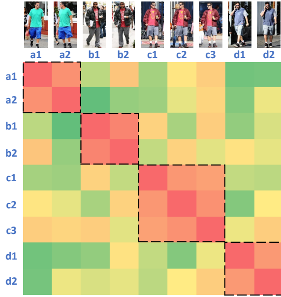
Figure 5.9 : Intra-class variation visualization using C-Caps. Four types of clothing (9 images) belonging to the same person (76 images in total) are selected in the training set of Celeb-reID. ‘a’ to ‘d’ represent different clothes and ‘1, 2, ...’ represents the index of sample images. The cosine similarity is used to calculate the similarity between two images using the VN capsules in C-Caps where the ID is presented. An activation map is used to represent the similarity between any two images. The red and green colors respectively represent the most and the least similar pairs. Elements in the diagonal are self-similar.
