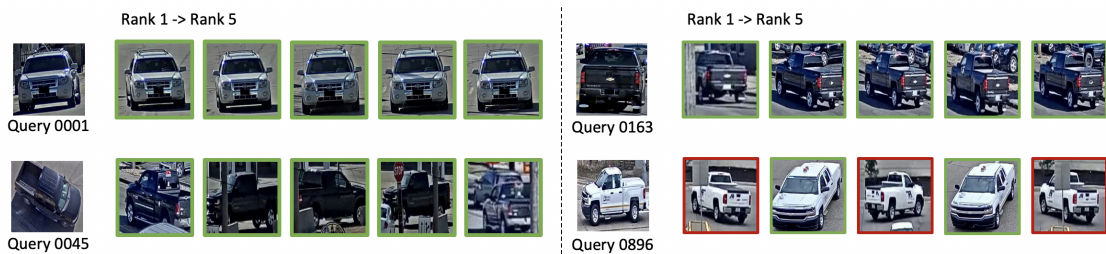
Figure 5.6 : Qualitative image search results using the vehicle query images from the CityFlow dataset. We select the four query images from different viewpoints. The results are sorted from left to right according to the similarity score. The true-matches are in green, when the false-matches are in red.
