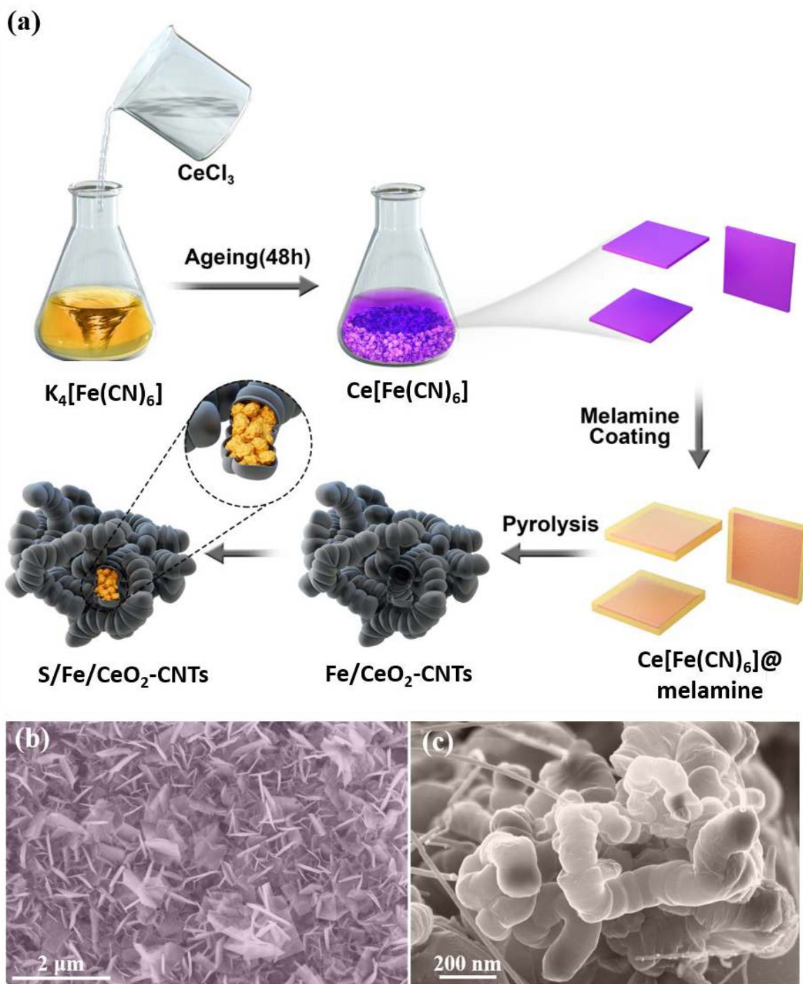
Figure 4.1. (a) Illustration of the synthesis process for preparing Fe/CeO 2 -CNTs hybrids. (b) SEM images of precursor Prussian blue analog nanosheets. (c) SEM images of the typical Fe/CeO 2 -CNTs structure after annealing at 900 °C.
