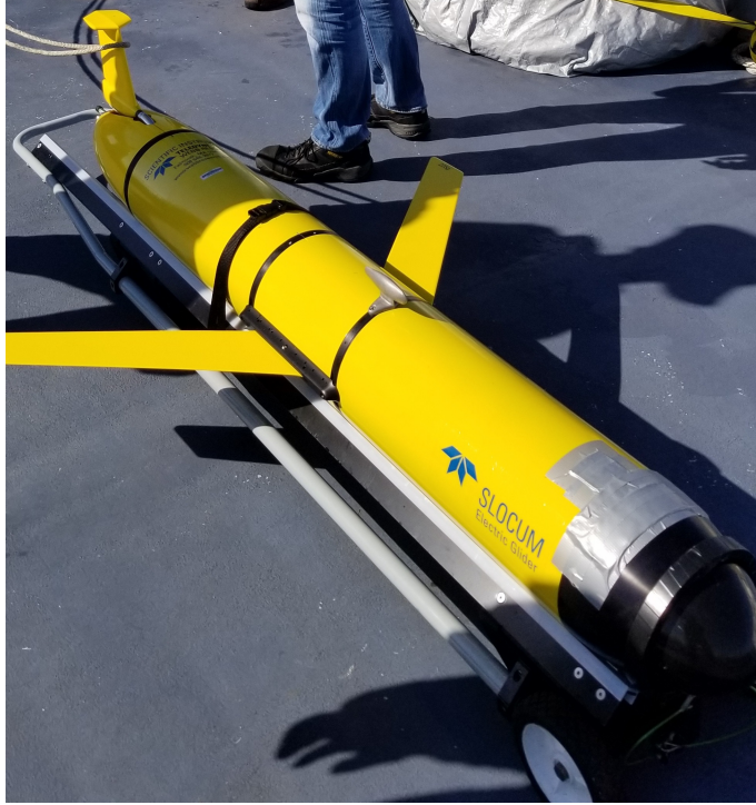
FIGURE 1.1: A Teledyne Slocum G2 underwater glider, deployed during many field trials.
