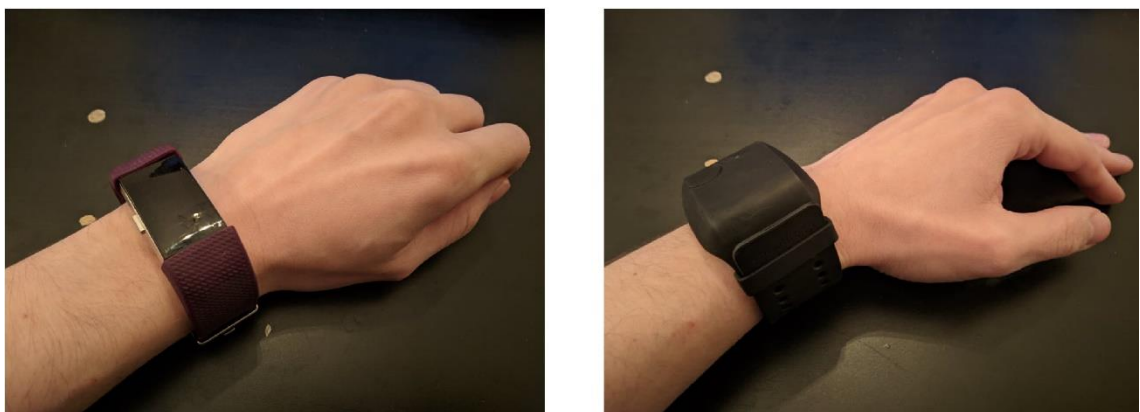
Figure 2.5. The wristbands used in the study (left: FitBit Charge 2; right: Empatica E4)
