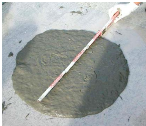
Figure 1.9 Measuring the diameter of flowability ECC of a slump flow test (Li 2008).
