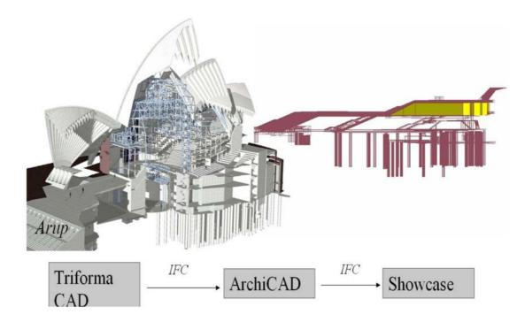
Figure 2.5 Using laser scanning to create 3D model of Sydney Opera House for facility management (Mitchell & Schevers 2005)
