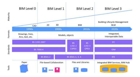
Figure 2.2 BIM maturity levels including codes of practice [BS...] following the UK BIM standards (Akbarieh et al. 2020)
