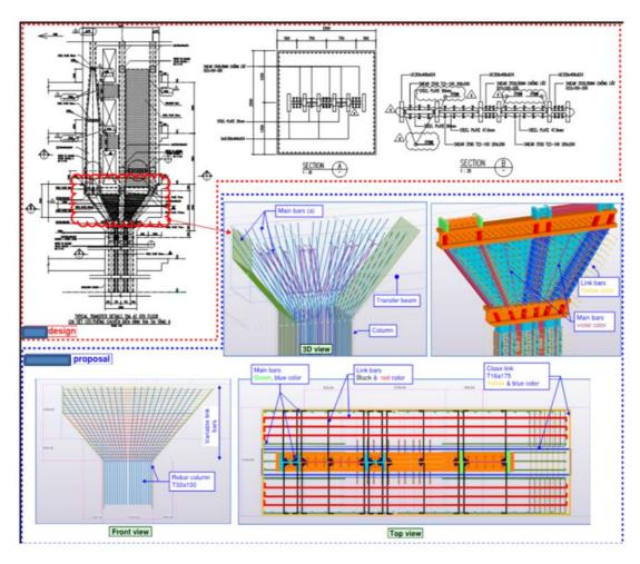
Figure 4.3 Transferring 2D designs to 3D shop drawings (by company C1)- Refer to Appendix 14 for full page figure
