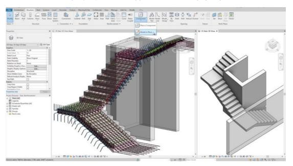
Figure 8.7 Less complicated stair component but commonly occurs at every floor (document shared by company C<sub>3</sub>)
