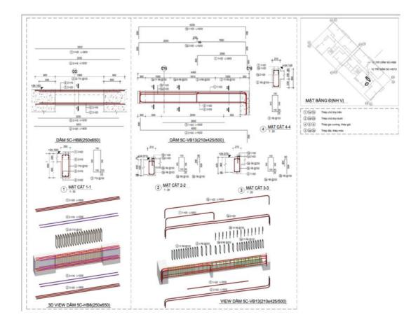
Figure 8.4 2D and 3D views of beam sections (document shared by company C<sub>3</sub>)- Refer to Appendix 19 for full page figure
