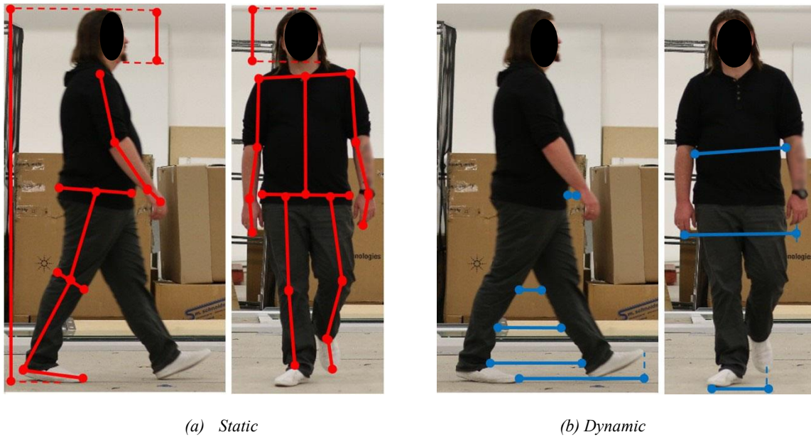
Figure 1.1 The Differing Types of Measurements/Proportions Analysed for Gait. The anthropometric measurements of the body (static and dynamic features) are applied for the assessment of gait. Static features (a) are defined as the geometrical measurements of the body, i.e. individual's length of whole leg, length of individual's knee to foot height etc. Examples of measurements taken are represented by lines. Dynamic features (b) are measurements related to gait. For instance, the distance between the left and the right toe during gait, distance between knees, stride length etc. The examples of such measurements are represented by the lines.
