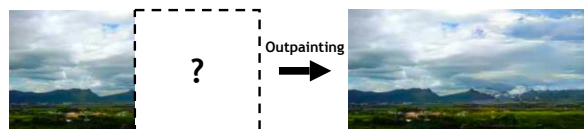
Figure 3.1: An illustration of one-step image outpainting, which predicts unseen contents outside the input region with the identical scale of the input. The semantic information and spatial layout must keep harmonious and consistent between predicted contents and the input scenario.
