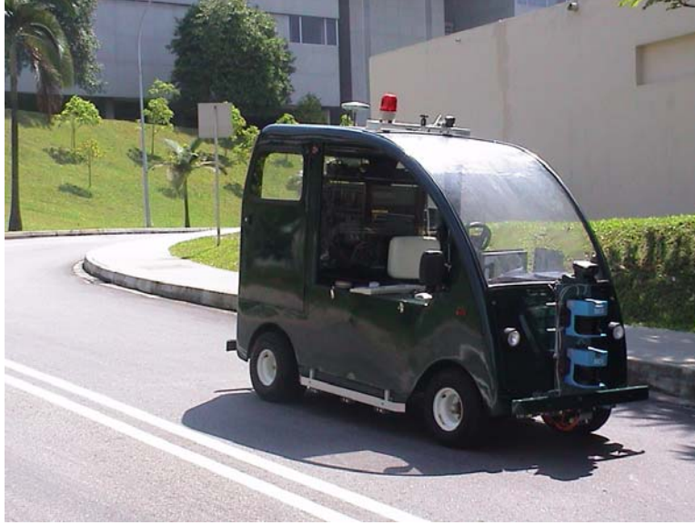
Figure 10: Laser/vision sensor assembly mounted on the GenOME
