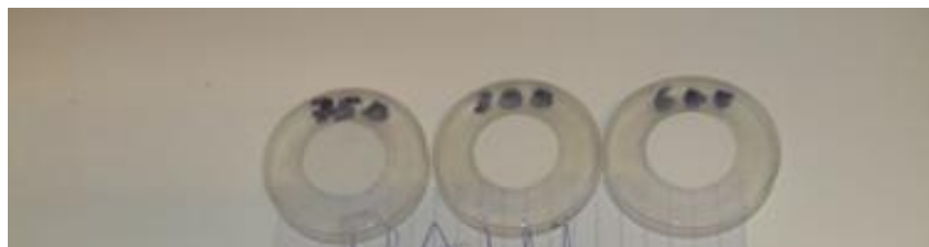
Figure 3.12 Prepared powder samples for XRD analysis
