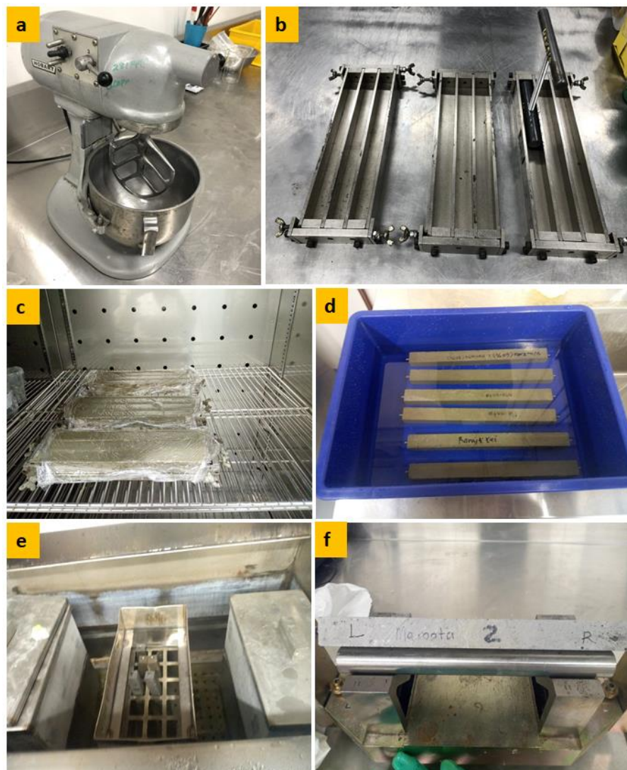
Figure 3.1 AMBT procedure showing (a) Horbat mixer (b) AMBT moulds (c) initial curing of mortar bars in a humidity cabinet (d) water curing of mortar bars at 80°C (e) ageing in 1M NaOH hot bath at 80°C, and (f) horizontal comparator for measuring expansion at respective ages
