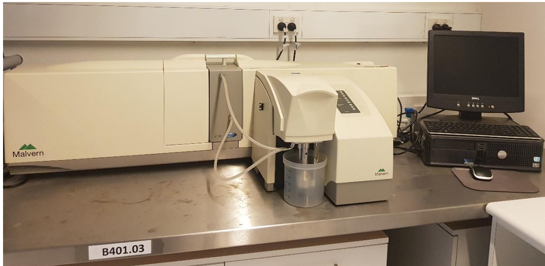
Figure 3.18 Malvern MasterSizer 3000 laser diffraction particle size analyser
