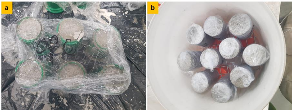
Figure 6.3 Photographs of paste specimens during curing phase for pore solution analysis
