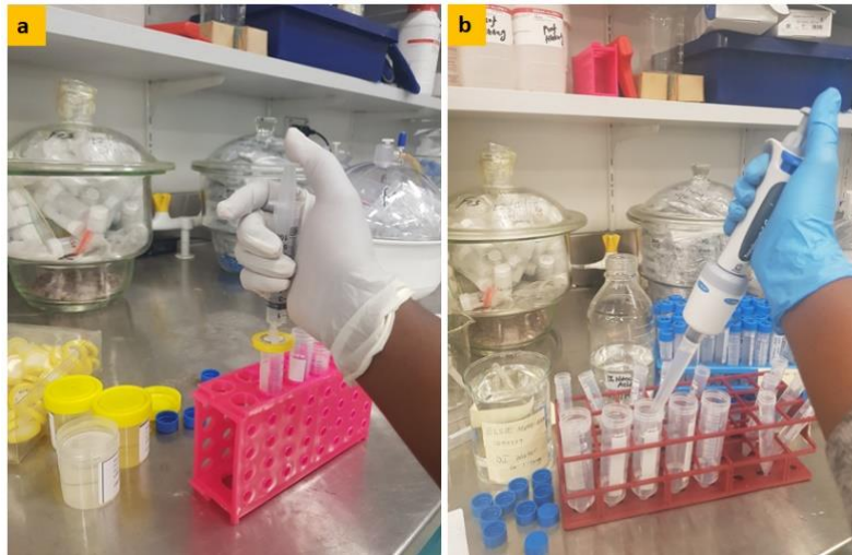
Figure 5.2 (a) Filtration and (b) dilution of sampled CPT and ACPT storage water for MP-AES analysis
