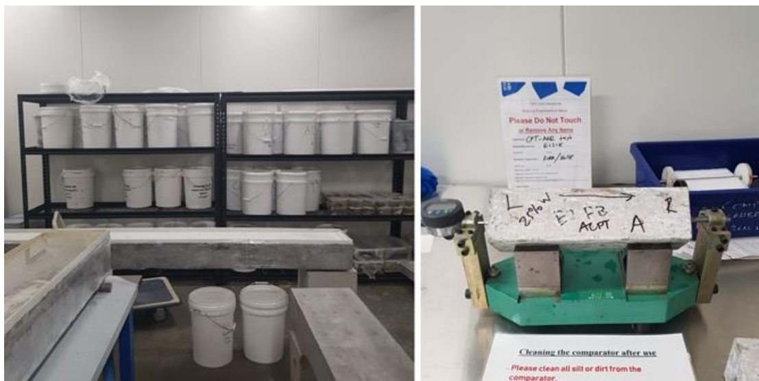
Figure 3.4 38°C environmental chamber for CPT and the horizontal comparator for CPT and ACPT prism expansion measurements carried out in this study
