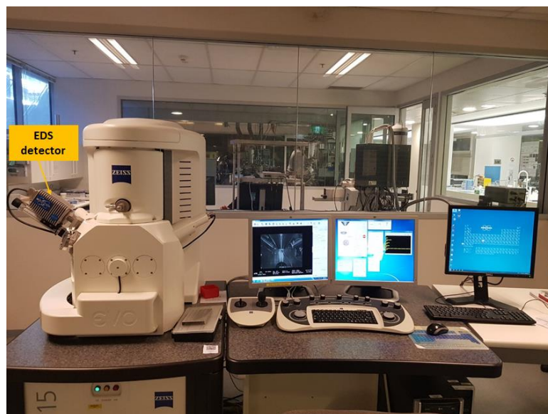
Figure 3.8 SEM-EDS instrument used in this study
