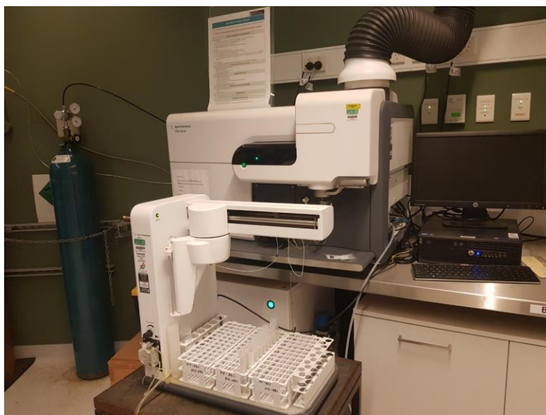
Figure 3.17 4200 Agilent Technologies MP-AES instrument with an autosampler
