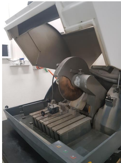
Figure 3.10 Labotom15 cutting machine for mortar and concrete sectioning
