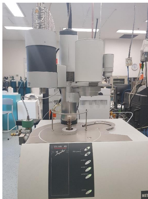
Figure 3.16 Thermal analyser used for TGA in this study
