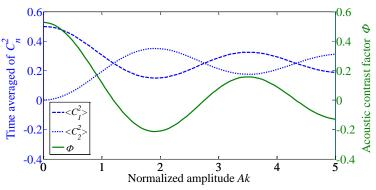
**Figure 2:** The acoustic contrast factor and  $\langle C_n(t)^2 \rangle$ , n = 1, 2 for different value of the Ak.
