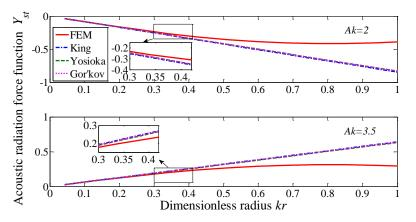
**Figure 3:** A comparison of the  $Y_{st}$  between numerical and analytical results for an oscillatory particle in a standing acoustic wave field over.
