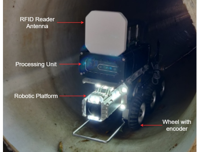
Fig. 1: Robot with RFID unit mounted on top.
