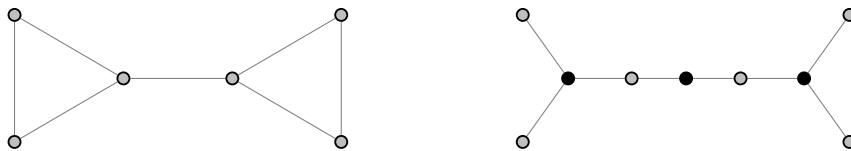
Figure 1: Example of a graph and its block-cut tree. Type II vertices are solid black.
