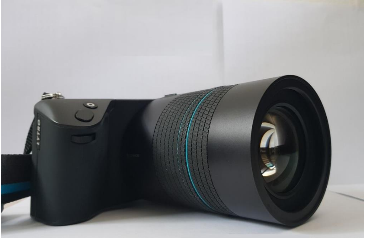
Figure 5. Lytro ILLUM Plenoptic Camera. In this thesis we used this Lytro ILLUM camera for some parts of our experimental results.
