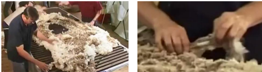
Fig. 1: The manual skirting process of contaminated wool fleece [1]. Left: Two wool handlers move along the edge of the fleece. Right: Close up of the hand position and gripping.
