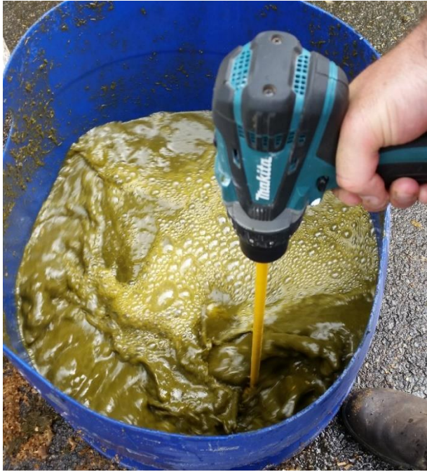
Figure 3.9. Total manure collected over 84 hours mixed with a measured volume of water using a paint stirrer.
