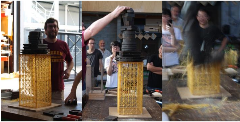
Figure 9. Pasta tower. Vertical load experiments to determine optimum diagrid dimensions to resist buckling.
