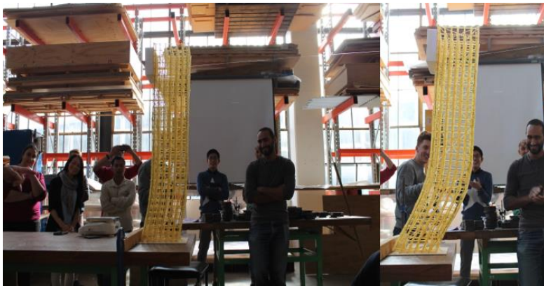
Figure 10. Pasta tower test. Towers made from pasta and built up to 1m height, to be tested laterally to simulate wind loading.
