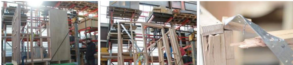
Figure 5. Half-scale wall testing. Typical walls built to AS1684 specifications. Left: Before test. Centre: During test with racking force applied. Right: Details of ruptured junction.
