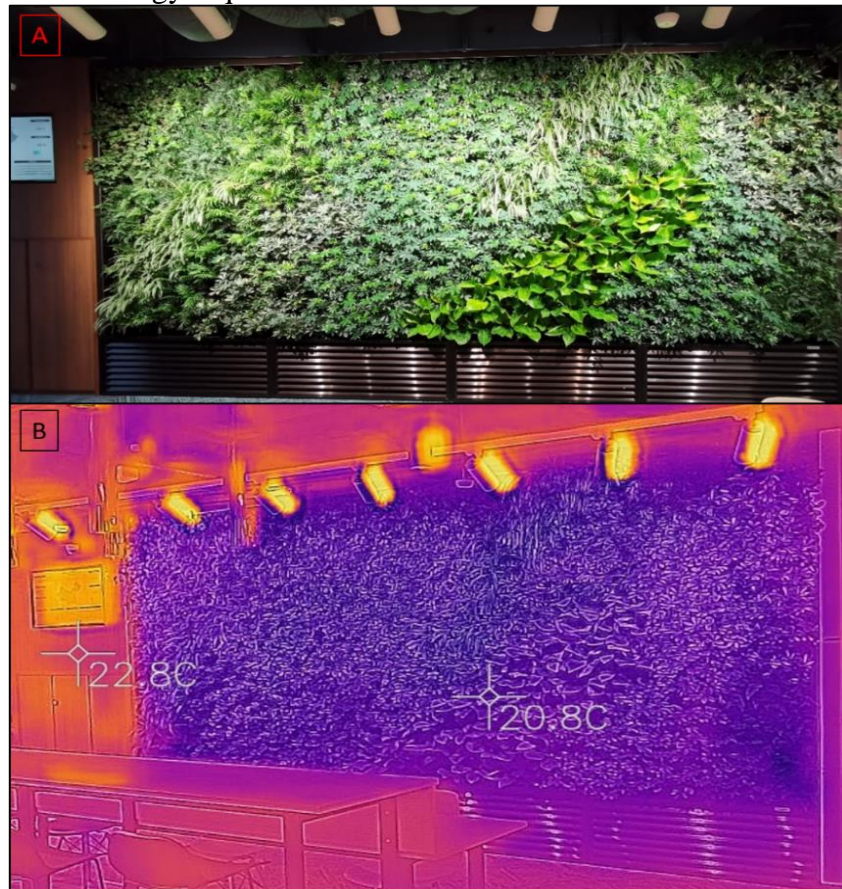
Figure 2: Bravolinear EnvoAir Active Green wall thermal regulation imaging (B). Source: Used with permission of Bravolinear Tech Limited.
