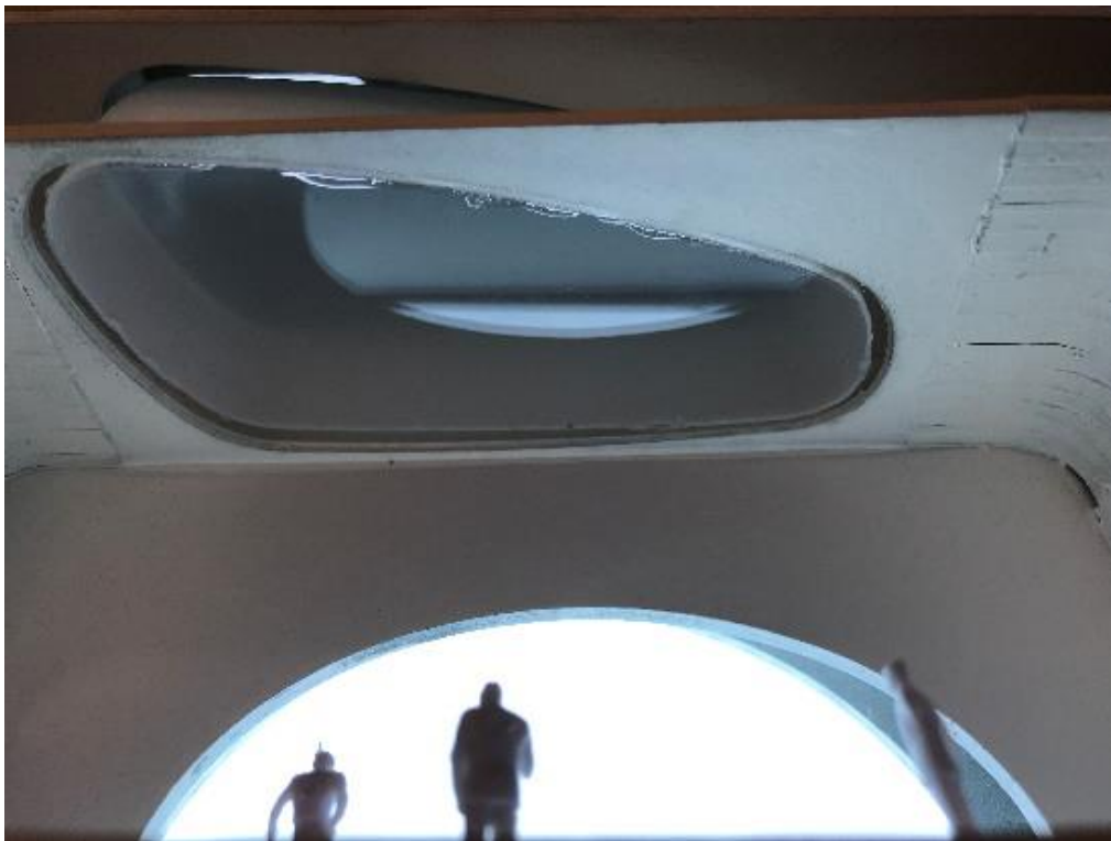
Figure 4.02 - An early model showing the south concourse with minimally defined cladding, yet the colour and wrap from wall to ceiling are already represented. Note that, even in this early model, the skylights from the octopus sketch have merged into a single skylight.
